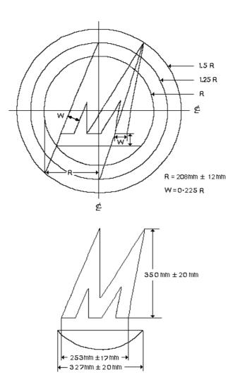
The dimensions are changed to W=0.225R minimum and 0.40R maximum. Height of M= 350mm+/- 25mm and the width of Half Moon M=327 +/- 65mm.
