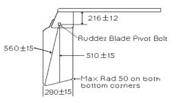
3.2 The dimensions of the **rudder** blade shall conform with the diagram. The **rudder** blade shall be not more than 14mm thick and the thickness shall not vary by more than 1mm to within 25mm of its edges with the exception of hollows or cavities of not more than 2mm in dimension and holes for fixing.
